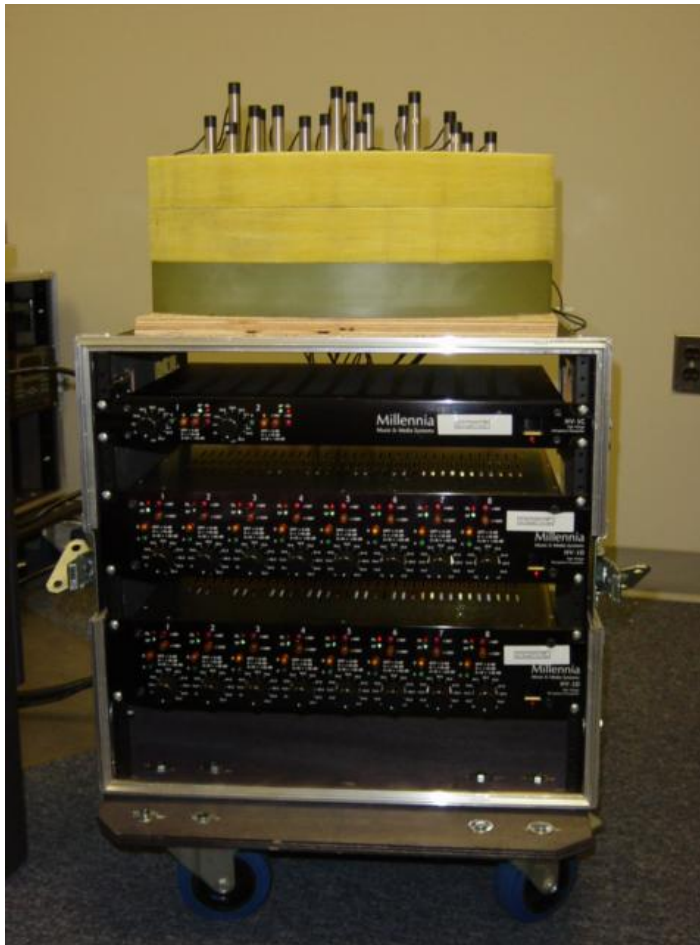
Air SPVA sensor and pre-amplifiers
