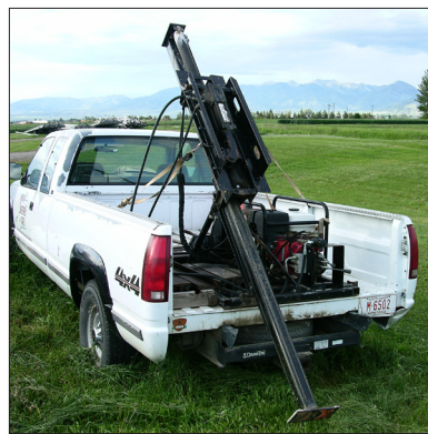
Figure 2. Soil sampling vehicle-mounted hydraulic probe.
