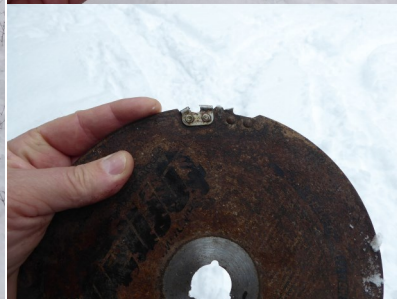
Picture 9. Thinning smaller seedlings and saplings can be accomplished most efficiently with a brush cutting head on a shoulder mounted “weed” trimmer. Different cutting heads have been developed for smaller diameter seedlings (top) or larger diameter stems (bottom) which feature chainsaw teeth. Cutting with a trimmer is best accomplished in spring and early summer when seedlings stems are softer— though many different cutting head styles exist for different applications. Cutting up to 3” diameter stems or larger is possible, but increasingly difficult to do as stems get larger and more woody.
