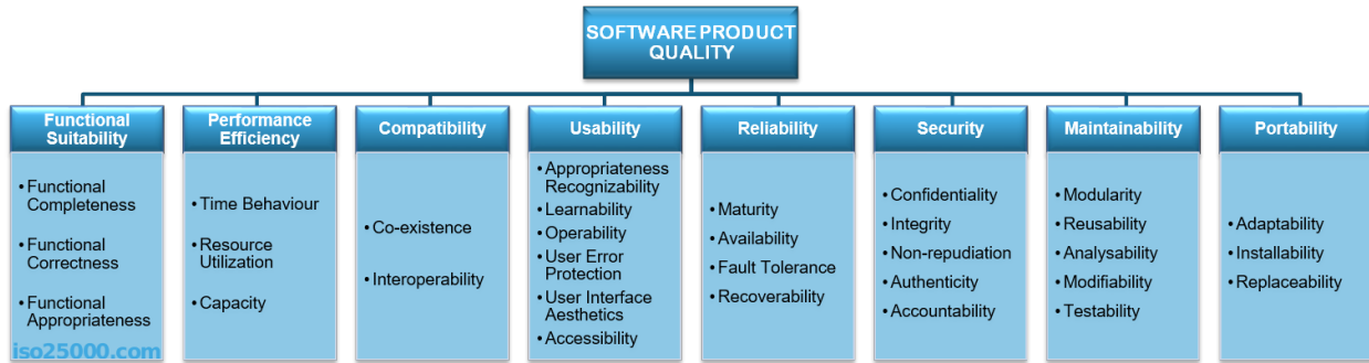
Figure 2.2: ISO/IEC 25010 Standard for Software Quality [20]. These eight attributes are meant to best represent stakeholder needs that can be included in a quality model.
