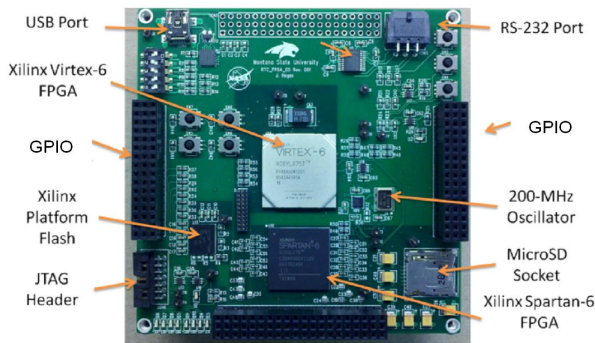
Fig. 1. Custom Virtex-6 Board Developed for the Benchmarking.
