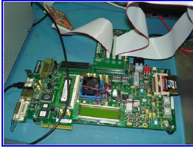
Fig. 8 Xilinx ML605 evaluation platform used to implement the 16-tile computer system.
