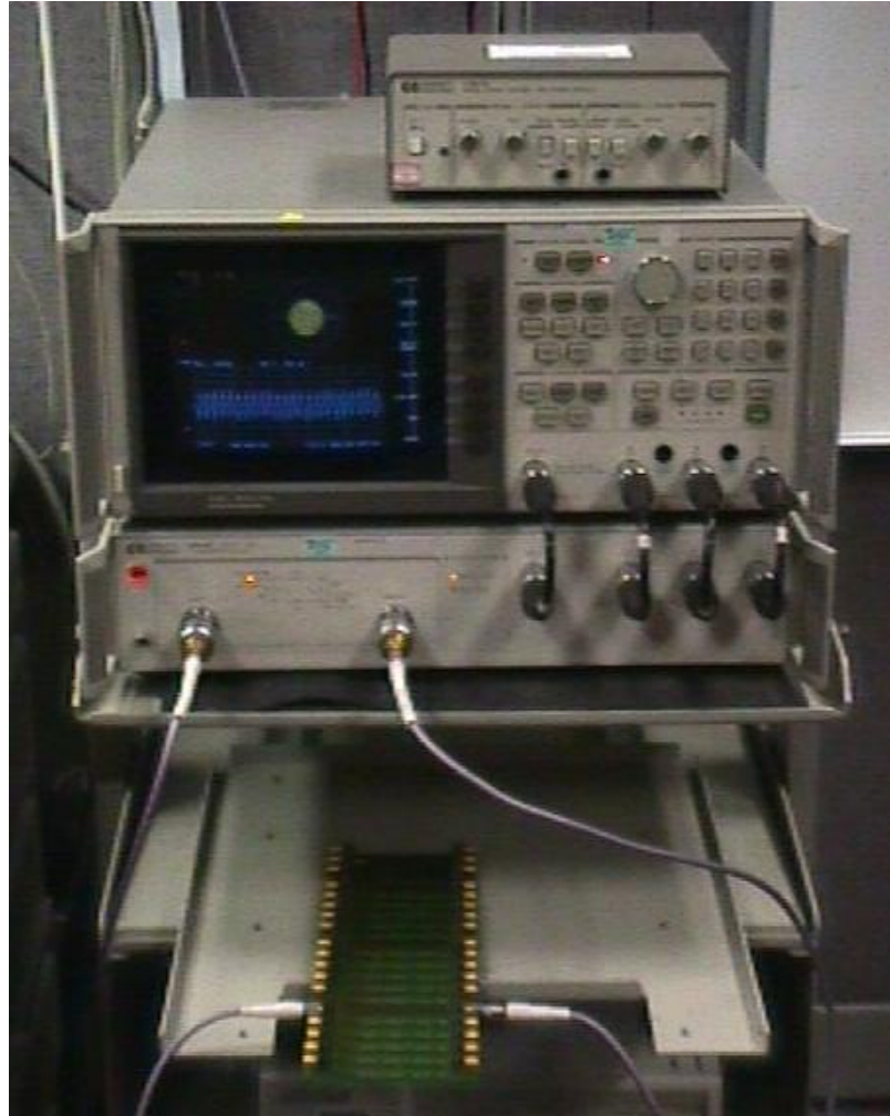
Figure 24. Laboratory Setup Used to Make Network Analyzer Measurements
