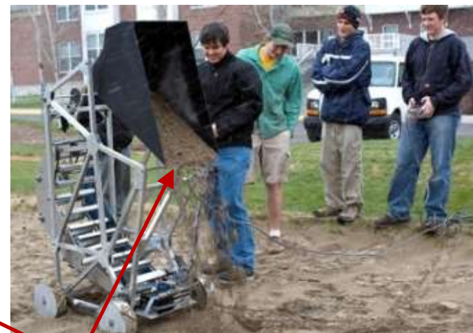
The hopper is shaped to dump over the edge of the sandbox.
