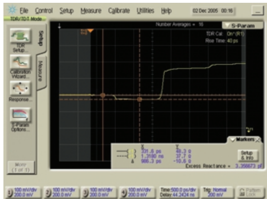
Figure 2. Using markers to measure the characteristic impedance of a transmission line.
