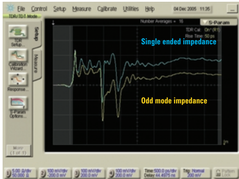
Figure 57. Comparison of the measured single ended impedance and odd mode impedance of a single line in a long motherboard trace.
